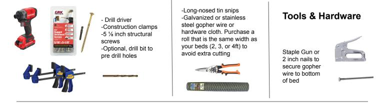
**3 ft x 8 ft Garden Beds:** Lumber is Pre Cut - Build on Flat Surface - Pre-Drill Holes before driving 5 1/8in Lag Bolts - Use Construction Clamps to secure 4x4 to 2x12 for Strong Fastening - Make sure beds end up the width of your gopher wire.
